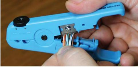
5. Insert wires into connector
